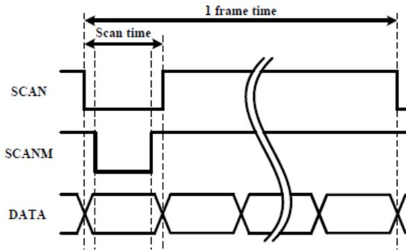
Fig. 2 Timing diagram of the pixel circuit
