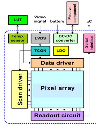
Fig. 5 Block diagram of driving circuit
