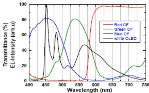
**Fig. 7 Spectrum of white OLED and color filter**
