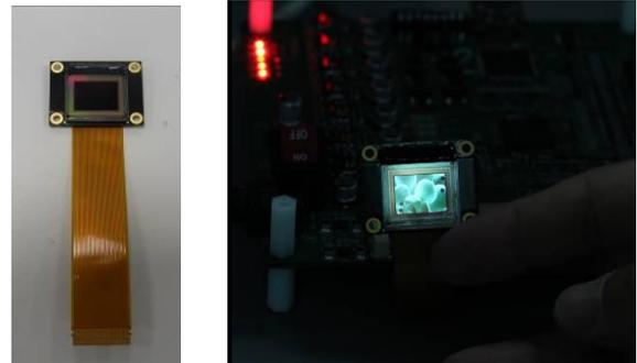
**Fig. 8 OLEDoS panel with flexible cable and OLEDoS panel driving with XGA image**
