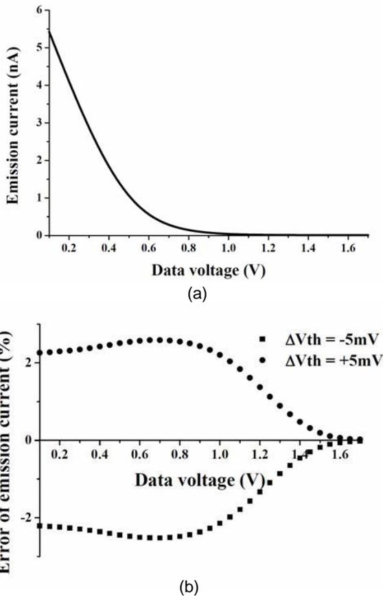
Fig. 3 Measured result of OLEDoS pixel circuit
