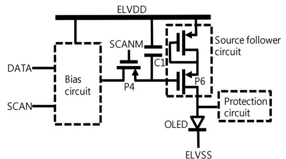
Fig. 1 Schematic diagram of the pixel circuit
